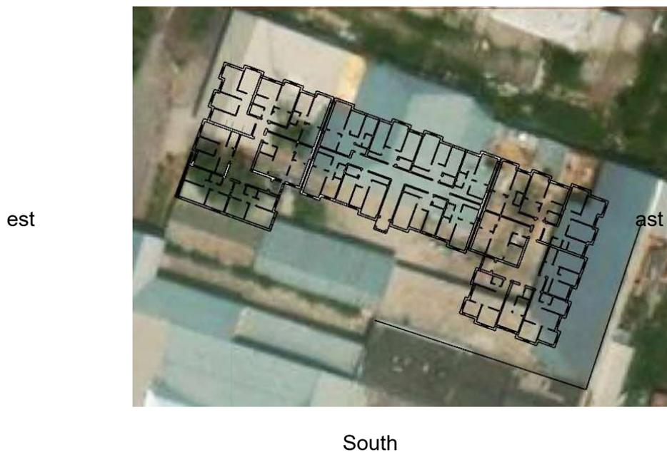
Figure 3. New building's sun insolation analysis using google map data. The old buildings on back side will be demolished. (Tashkent LAT: 41.350623° N LON: 69.222024° E)
