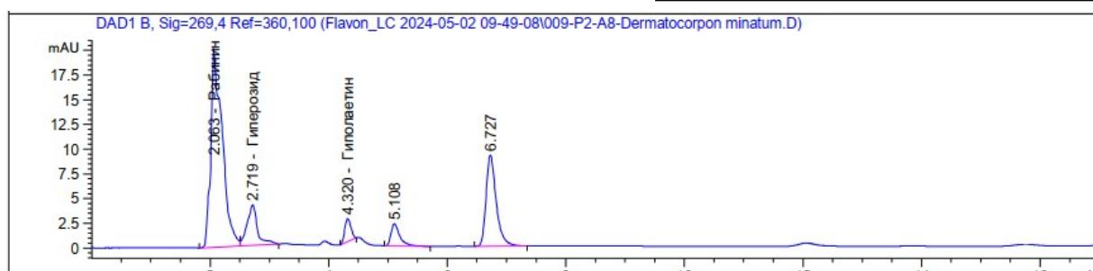
**1-rasm. *Dermatocarpon miniatum* lishaynigi flavonoid tarkibi xromatogrammasi**
