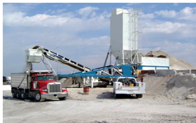
Figure 4. a) Mixing plant b) loading to dump truck
