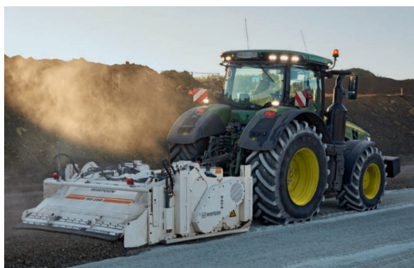
Figure 3. a) tractor-towed stabilizer, b) working process
